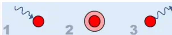
Fig. 1: Light reflection on a surface: Light falls on an atom (1), which absorbs the energy and is thus excited (2), and then emits the energy again.
