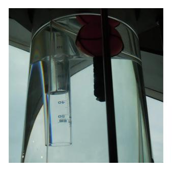
Use the lever to pump air into the large cylinder.
