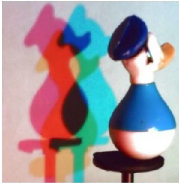
Fig. 3: Additive colour mixing in penumbras.
