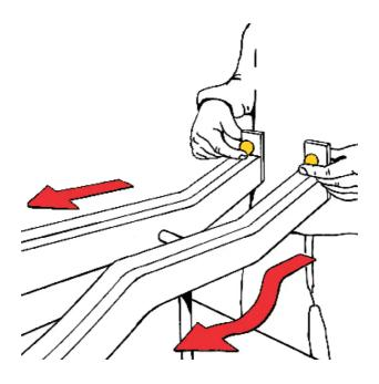
Place both balls on the highest point of the track. Let both balls go simultaneously. The ball running through the hollow detour arrives earlier than the ball travelling on the straight connection.
