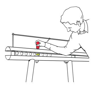
Hold the black magnet above the copper slab, directly over the silver magnet. The silver magnet doesn't fall straight down – it moves as if it is in a very thick liquid.
