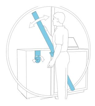
Turn the valve to "air" to let air into the plastic cylinder.
