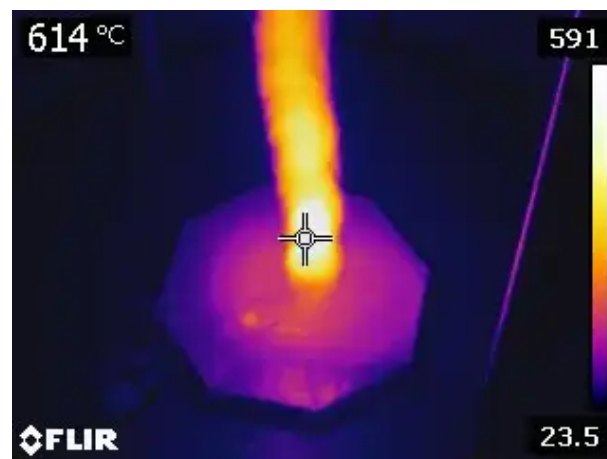
Fig. 1: Fire-tornado temperatures recorded with an IR camera. The colours depict the temperatures in °C.
