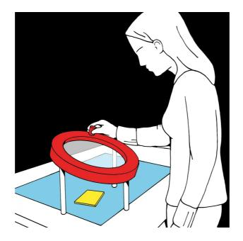
Rotate the disc using the red handle until the light seems to be dim.
