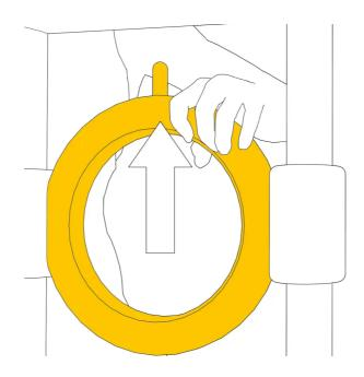
Slide the metal ring to the top of the frame.
