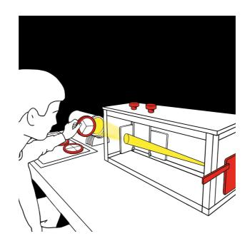
Put different combinations of filter discs in the holder by the lamp.
