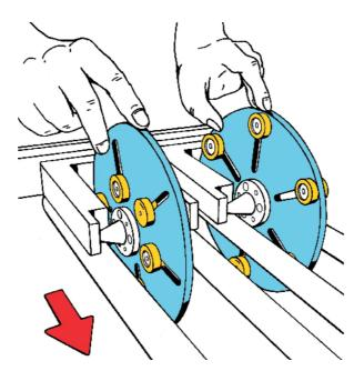
Put two disks of the same weight on the slope and observe them rolling down. For each weight there is one disk where you can shift the small weights.
