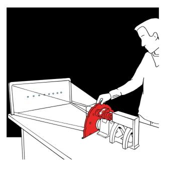
Turn the wheel slowly to move one of the ten openings between laser and projection wall and watch the resulting light patterns.
