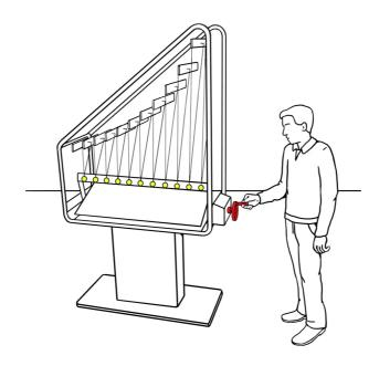
Turn the handwheel until the pendulums are released and begin to swing.
