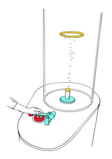
Push down the lever on the red bellow to press air into the water cylinder .
