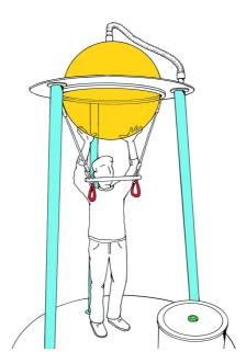
Push the green button to start evacuating the air from the Plexiglas sphere.
