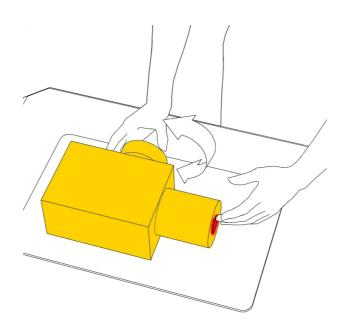
Notice that when you turn the knob, a plunger moves in and out of the end of the metal cylinder.
